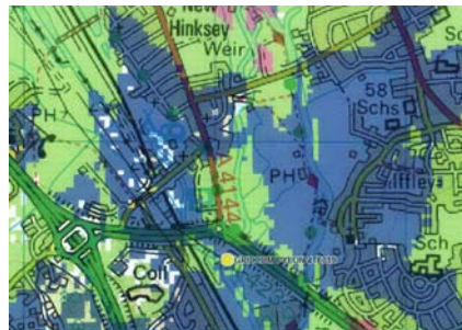
Figure 3: Coverage plot where blue areas represent low ('outdoor only') levels of network coverage
